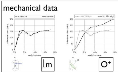
We conducted a series of deformation experiments at conditions where dislocation glide is active ( $T = 900^\circ\text{C}$  and  $1000^\circ\text{C}$ ,  $P_c = \text{of } 1 \text{ to } 1.5 \text{ GPa}$ ,  $\dot{\epsilon} = 10^{-6} \text{ s}^{-1}$ ).
