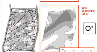
Whole samples (left) and maps of water content, FTIR measurements (right). In 144 samples, the occurrence of the peak at  $3582 \text{ cm}^{-1}$  is restricted to the barrel shaped bottom part; in O+ samples, they occur everywhere.
