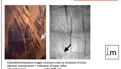
Cathodoluminescence images: contrast is due to variations of trace element concentration = indication of water influx
